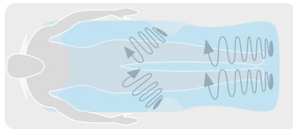
The authentic Jacuzzi® hydromassage has jets inclined at 30°, which can be positioned in any direction.
